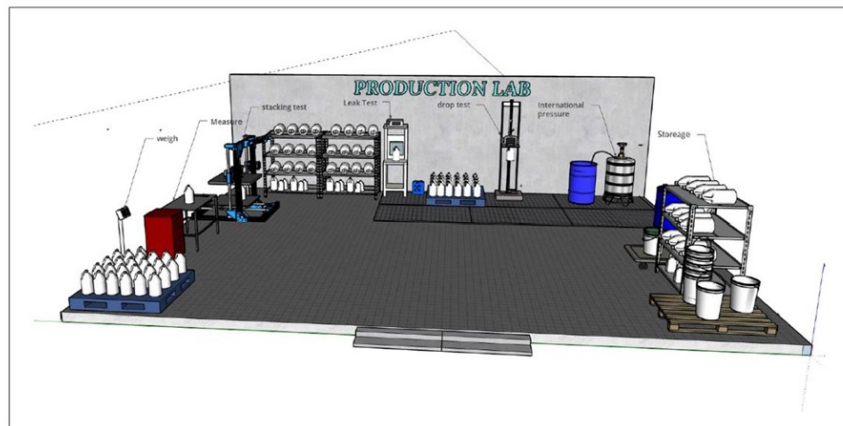
Performance Testing Laboratory for Packaging Containers
