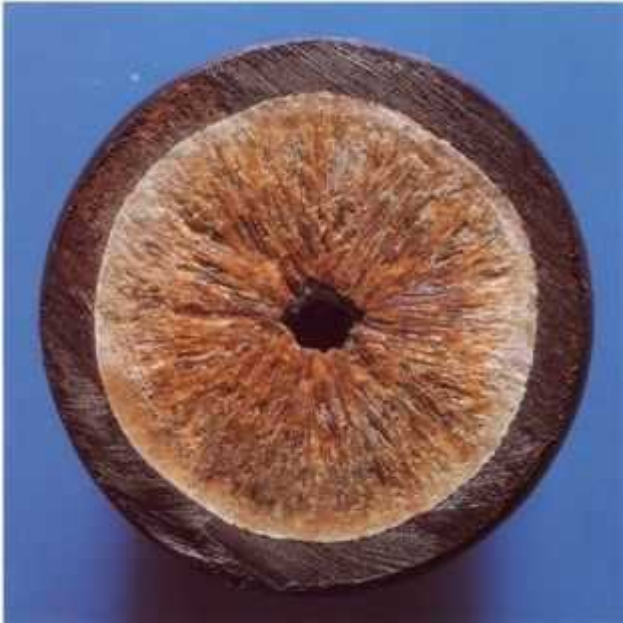
Galvanized pipe heavily scaled
